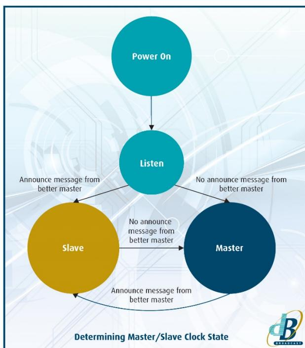
Once a master is established, it sends sync and follow-up messages that are used by slaves to begin to derive the time. Although it is easy for the slave to determine the propagation delay from the master to the slave, the slave also needs to know the reverse path delay. This is achieved by the slave sending a Delay Request message to the master. Once received by the master, it time-stamps the time of receipt and sends this back to the slave as a Delay Response message.
