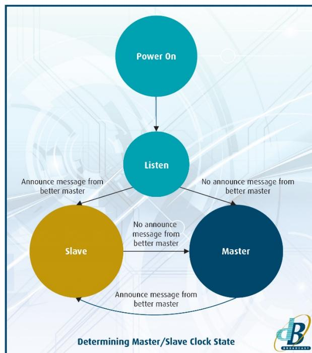
Once a master is established, it sends sync and follow-up messages that are used by slaves to begin to derive the time. Although it is easy for the slave to determine the propagation delay from the master to the slave, the slave also needs to know the reverse path delay. This is achieved by the slave sending a Delay Request message to the master. Once received by the master, it time-stamps the time of receipt and sends this back to the slave as a Delay Response message.
