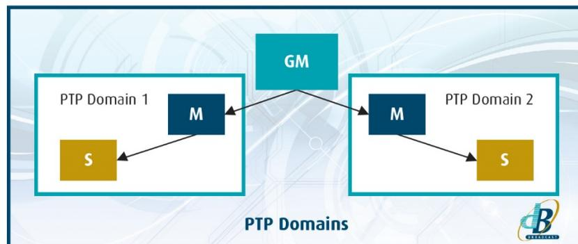
Clocks in one domain may not necessarily be synchronised to clocks in another domain, although in a broadcast network it is typical to have all domains synchronised to a single grandmaster.
